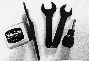
Fig 1: Tool kit - vaseline, toothbrush, ADE spanner set, screwdriver
